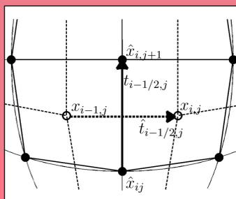
The angles in the discrete finite volume formula are the angles between primal (solid) and dual (dashed) vectors.
